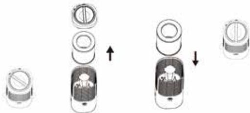
3. Align the arrow on the cap with OPEN on the unit and screw it in towards the CLOSE position.
