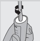
**2** Insert a screwdriver into the slot located at the bottom of the handle and turn counterclockwise to release the bottom cap.
