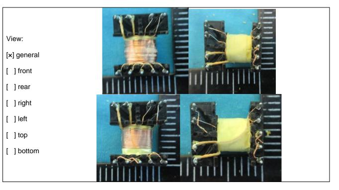
Details of: Transformer(QH1605V001) : Triple insulated layers wire
