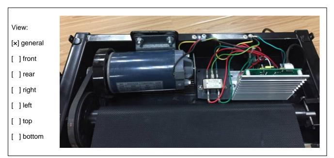
Details of: Electric part view after removing the guard
